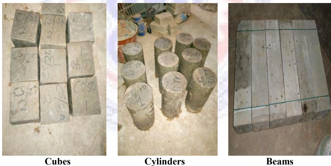
Figure 3.13: Samples of specimen arranged for visual inspection
