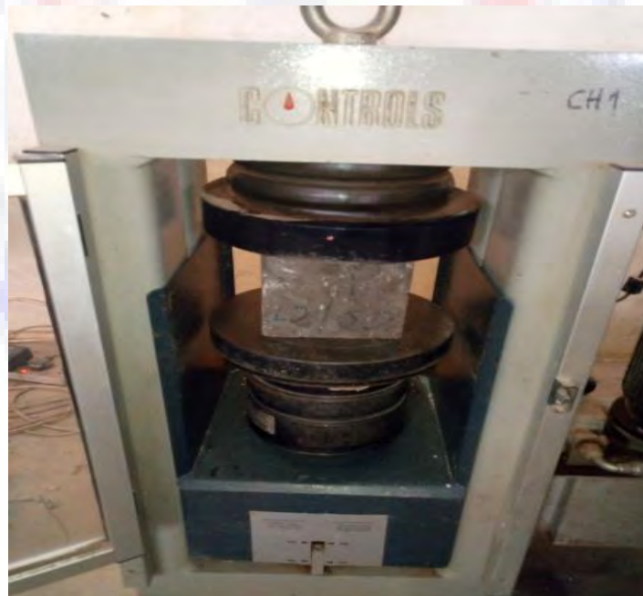
Figure 3.14: Compressive Strength test set up
