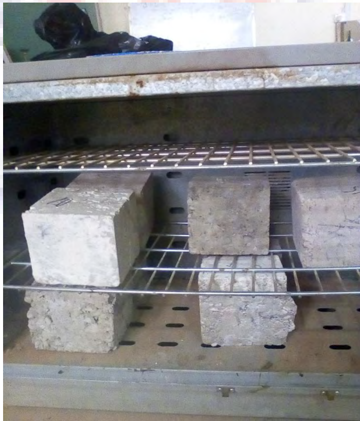
Figure 3.7 Cubes in the oven
