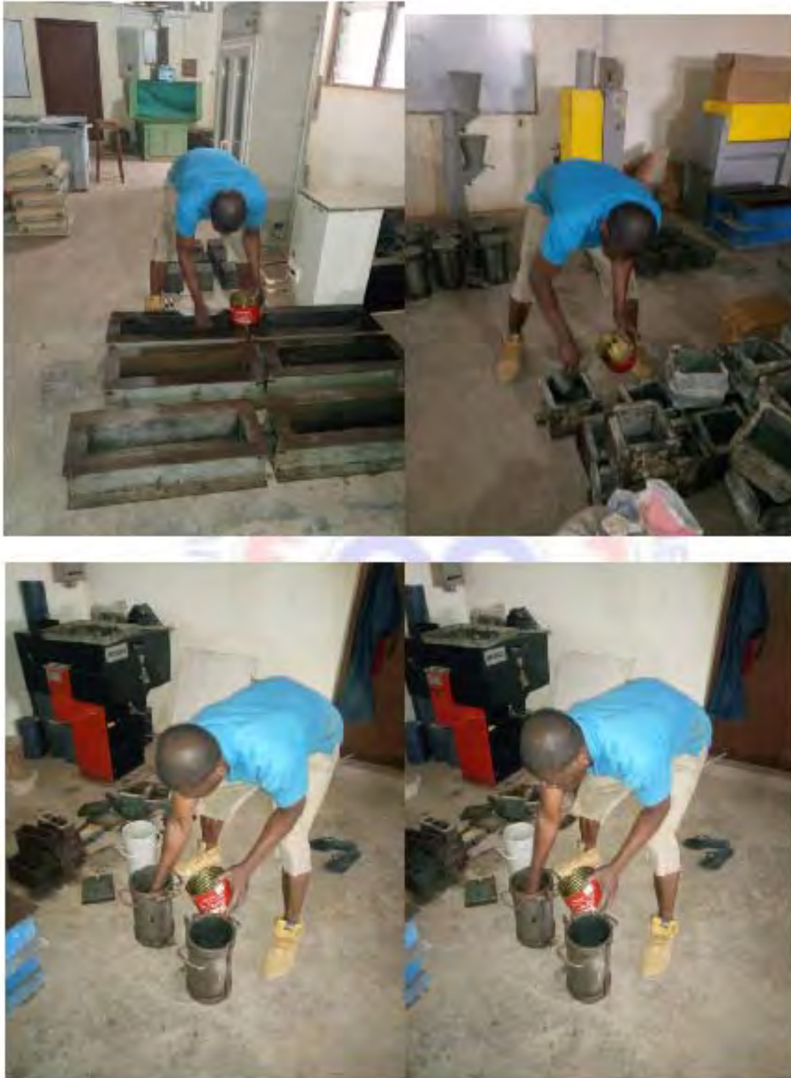
Oiling of concrete moulds
