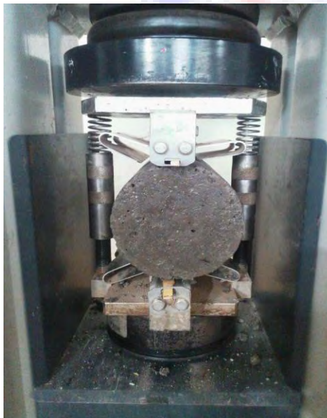
Figure 3.5 Before splitting of cylinder
