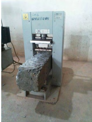
Figure 3.3 Before flexure of prism Figure 3.4 After flexure of prism
