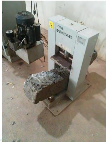
Figure 3.3 Before flexure of prism Figure 3.4 After flexure of prism
