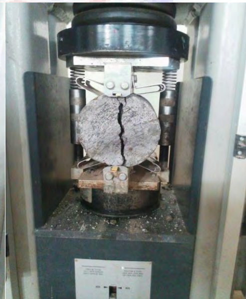
Figure 3.6 After splitting of cylinder
