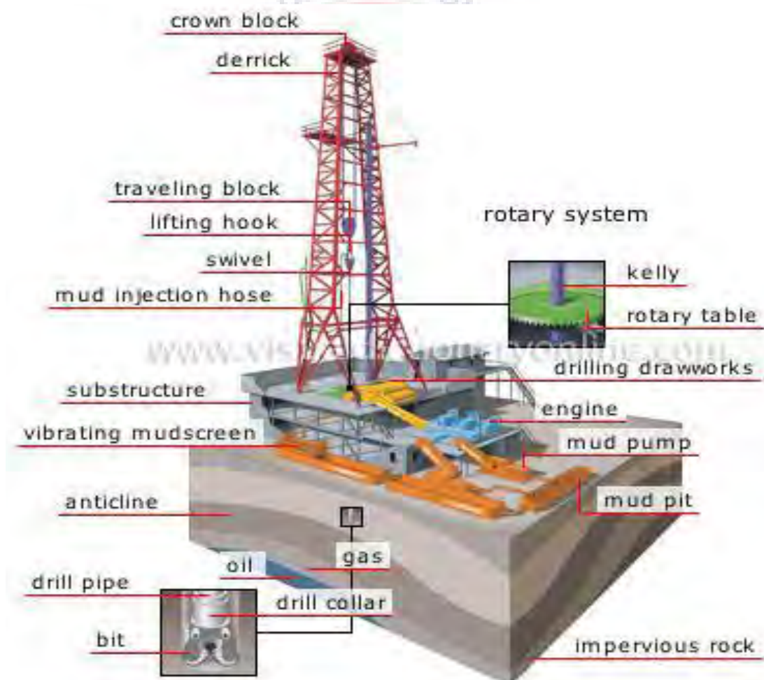
Figure 2: Drilling Rig setup
